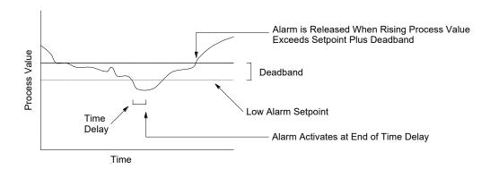
The illustration above shows the action of a low alarm setpoint on a falling value.
