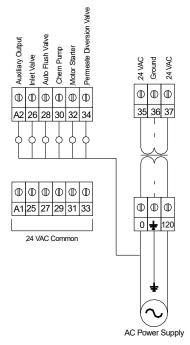
The solenoid coils are referenced to high voltage power supply.
