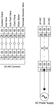
The outputs are referenced to 24VAC after the 24 VAC transformer.
