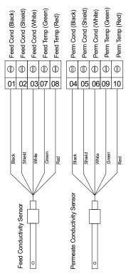
NOTE: Terminal numbers are not in order intentionally. This allows terminal connections to match previous versions of the controller.
