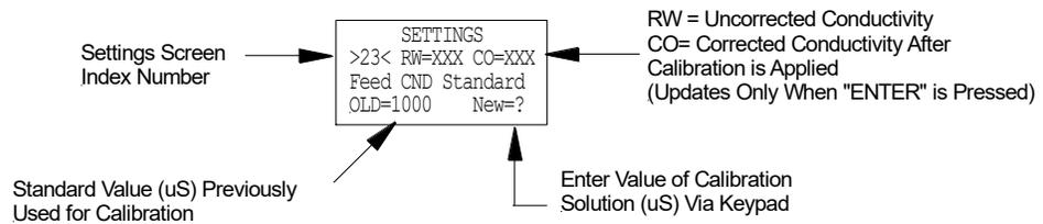
If the value displayed on the screen does not match the value entered for the calibration solution, let the sensor equalize for a few more minutes and repeat Step Two.
