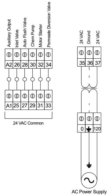
The outputs are referenced to 24VAC after the 24 VAC transformer.
