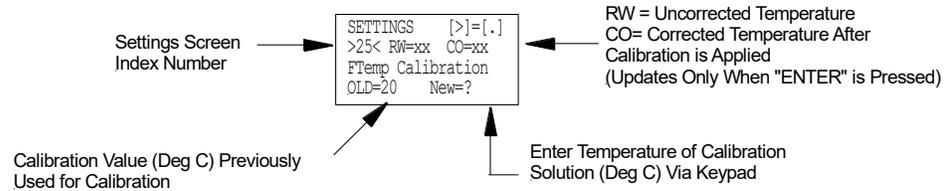
If the value displayed on the screen does not match the value entered for the calibration solution, let the sensor equalize for a few more minutes and repeat Step Two.
